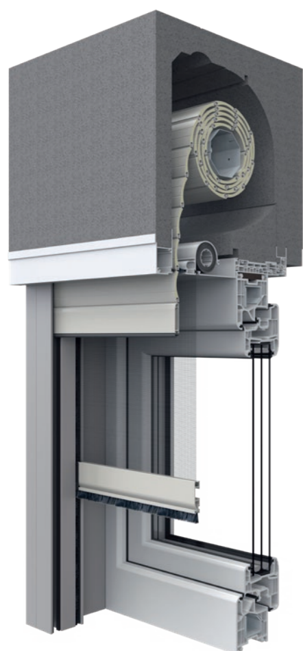
TOP FOAM RvA With integrated recess to incorporate roller shutters, inspection from the outside, optionally with insect screen.
