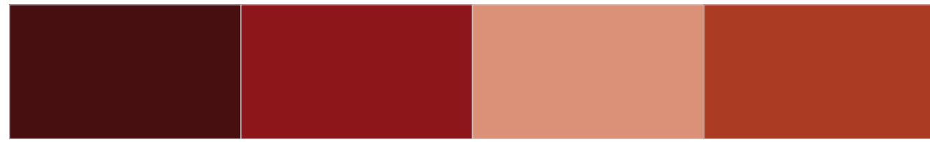
RAL 3009 Oxide red RAL 3011 Brown red RAL 3012 Beige red RAL 3013 Tomato red
