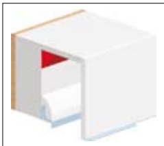
Insulation wedge with installation of roller shutters
